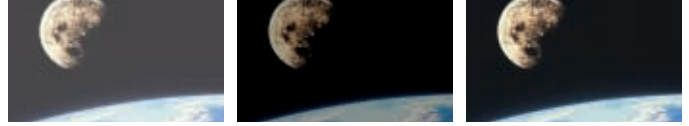
Without lamp power control or dynamic gamma correction blacks and other colors appear lifeless.
