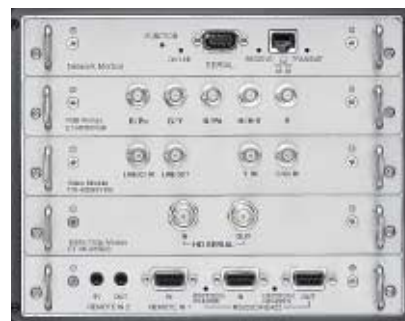
Two sets of terminal boards (network and remote control) are supplied. Up to three optional boards can be installed.
