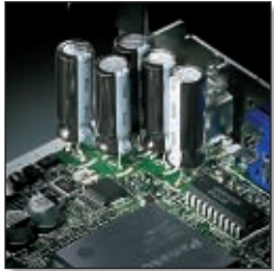
Separate power supply for cooling fan and control circuit
